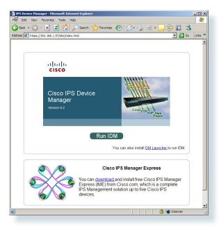
Since we are configuring several sensors in this network, we want to use Cisco IME (IPS Manager Express). It allows for management and monitoring of up to 5 IPS sensors from a single application. To download IME, go to the IPS initial webpage and the link provided to install on your local machine now. Next, launch IME and you should see the starting IME home screen. To add a sensor, click on the **[add]** button under devices.
