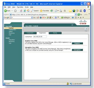
Step 3: Enter IP address of the WAAS CM and click on Register.
